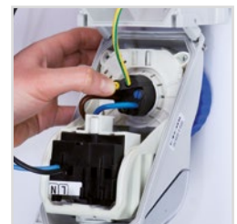
Screwless earthing conductor connection, max Ø 4mm; ~ 10 mm on 32 A.
